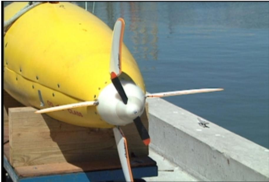
The Dorodyssey vehicle maneuvers using a propeller and fins.
