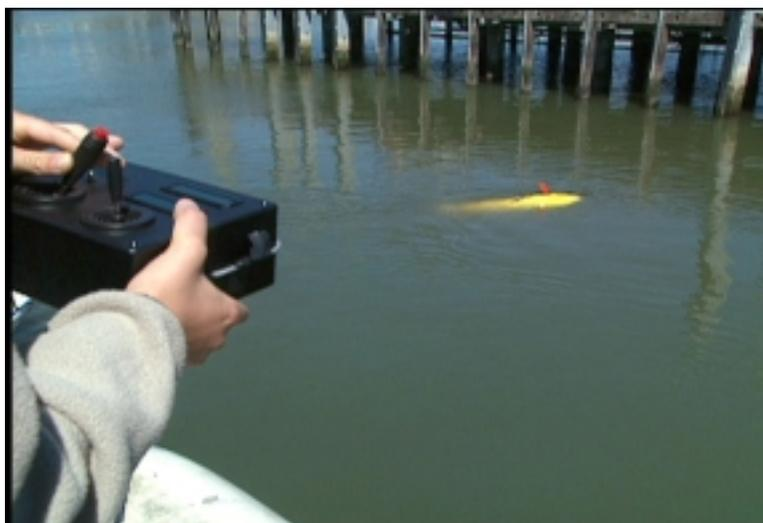
A manual control lap box allows an AUV to be controlled at the water's surface.
