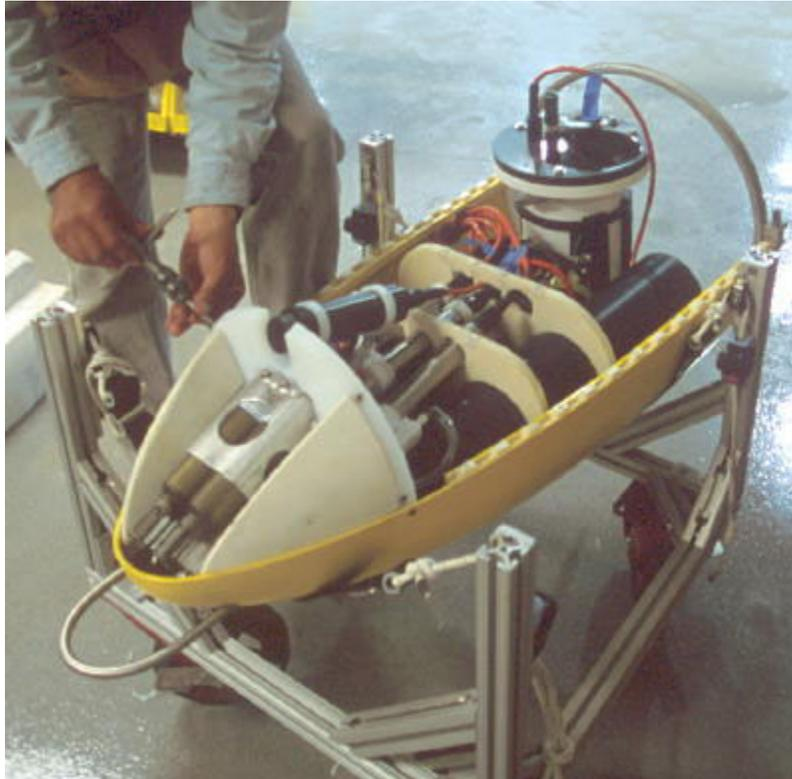
Figure 1: The scientific payload of the AUV is mounted in the nose section. The space above the components is taken up with syntactic foam when the vehicle is fully assembled.
