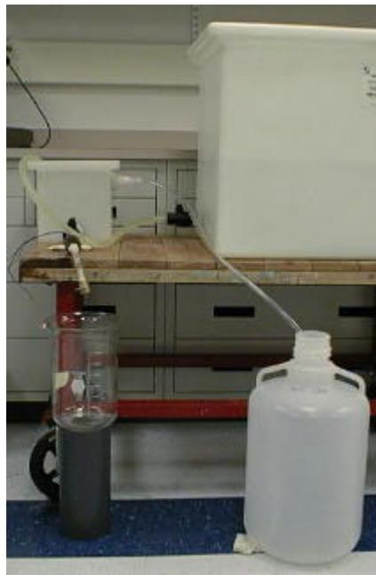
Figure 4: A constant-flow apparatus was assembled to characterize the frequency response vs. flow rate for each flow sensor.
