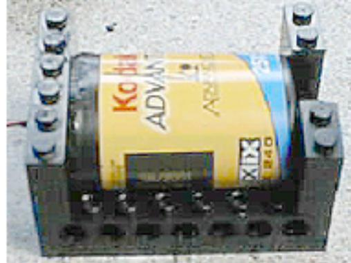
Figure 4: Finished Waterproof Motor in LEGO brace
