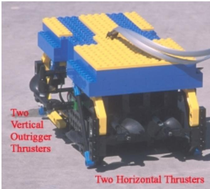
Figure 6: Thruster Configuration
