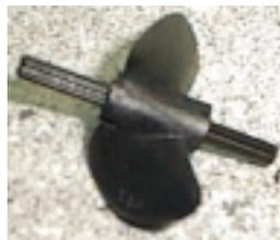
Figure 5: Prop Glued onto LEGO Axel
