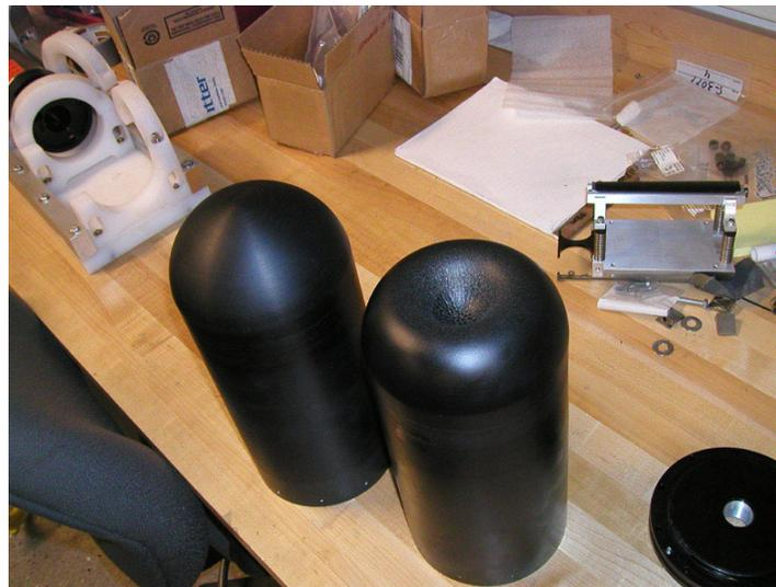
**Figure 1 Originally Identical Aluminum Objects; the right one failed pressure tests**
