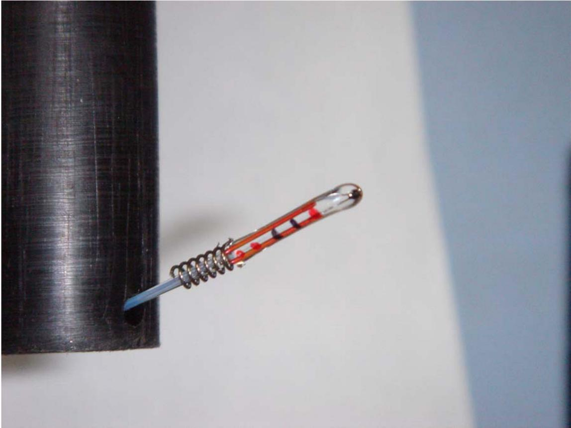
Figure 5: Thermistor, compression spring that sits behind thermistor, and Teflon insulation around downstream lead of thermistor (not the Vref lead) shown before being sleeved into mounting hole in Delrin rod.
