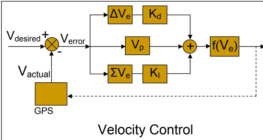
**Velocity PID Control Loop.** PID is a standard error driven control method.
