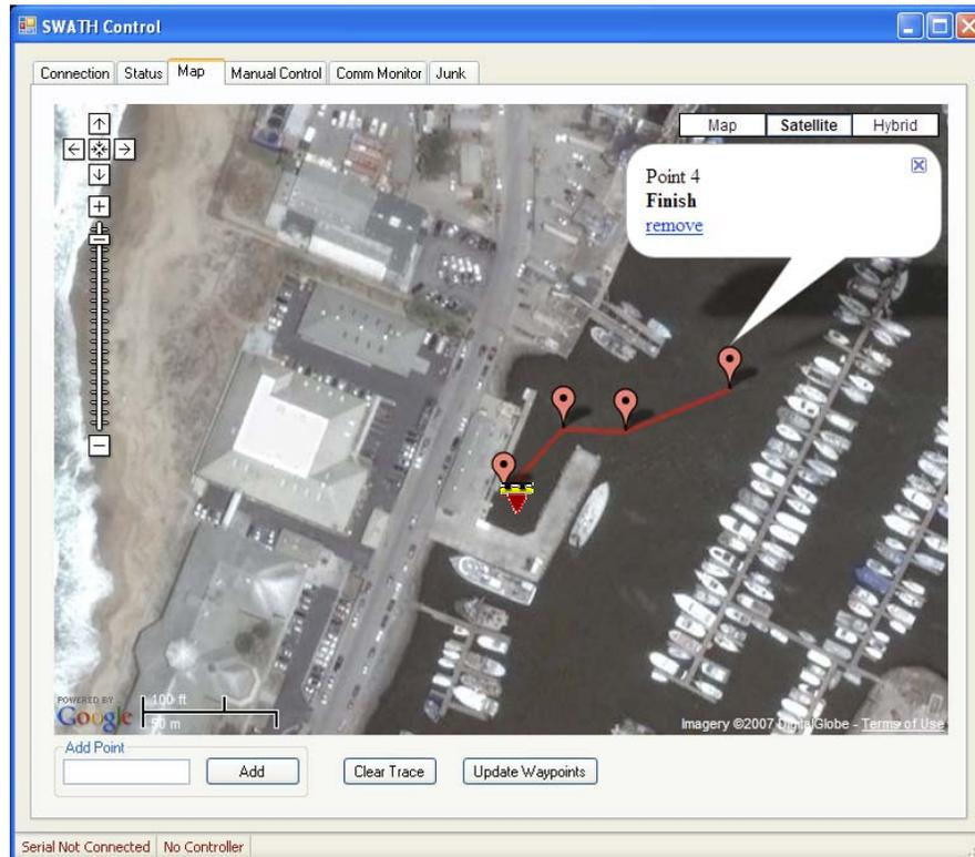
**Google Maps Interface.** Using C# hooks into javascript, Google Maps was able to be utilized for real time monitoring and waypoint routing for the autonomous SWATH boat.
