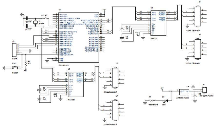
**Circuit diagram for the main controller.** A single PIC microcontroller contains all the abilities to perform complex communications and PID control. There are four serial ports used for communication among devices.
