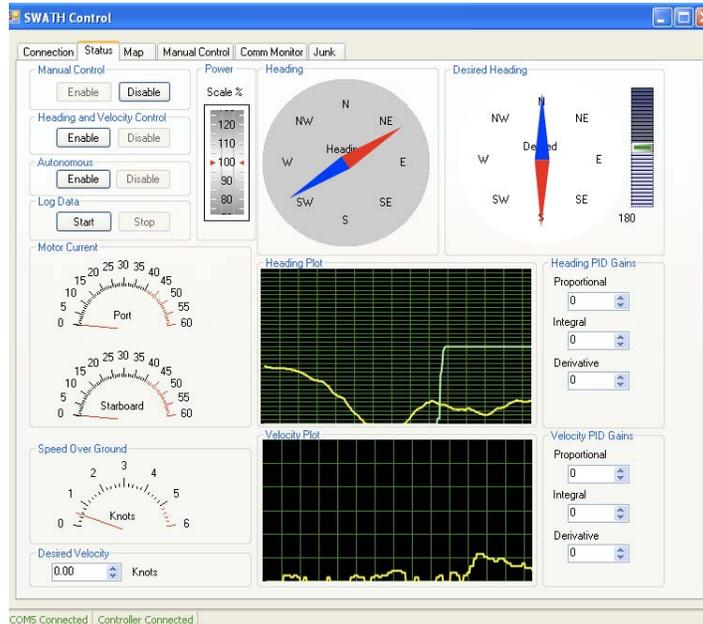
**Monitoring Graphical User Interface.** The graphical interface designed in Microsoft Visual C# allows monitoring and adjusting the boats performance, including tuning PID gains in real time.
