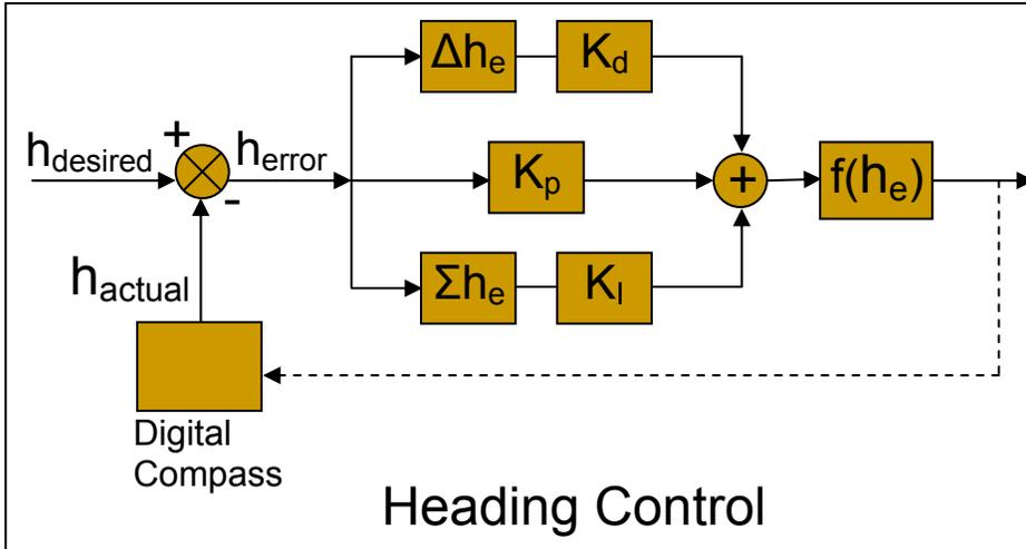
**Heading PID Control Loop.** PID is a standard error driven control method.
