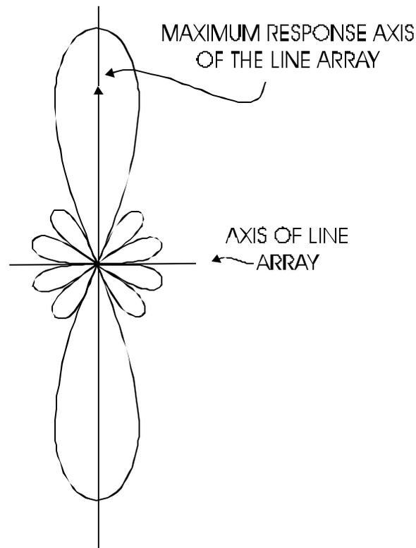
**Figure Chapter 3 - -15: Beam Pattern for a Line Array of Hydrophones**
