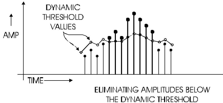
**Figure Chapter 4 - -24: Eliminating Amplitudes Below the Dynamic Threshold**
