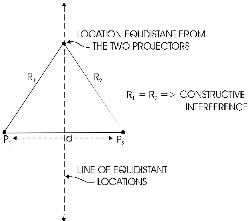
**Figure Chapter 3 - -3: Positions of Constructive Interference (Example 1)**
