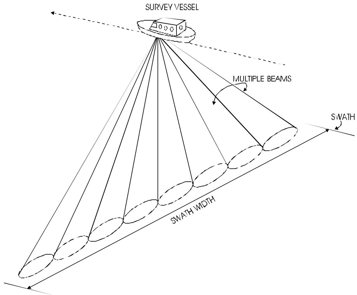
**Figure Chapter 2 - -9: Multibeam Sonar Swath**
