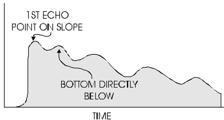
**Figure Chapter 5 - -15: Amplitude versus Time Plot for the Situation Depicted in Figure Chapter 5 - -14**
