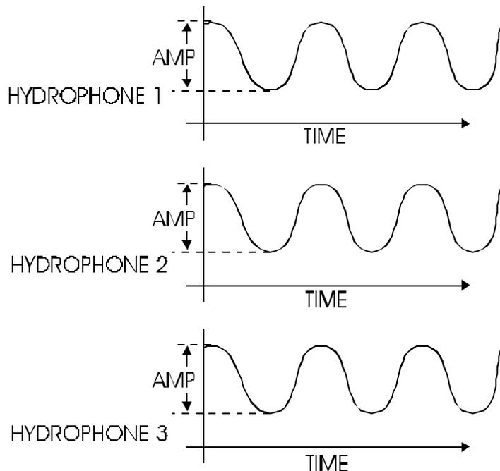
**Figure Chapter 3 - -10: Hydrophone Traces for a Perpendicular Source**
