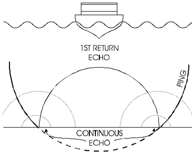
**Figure Chapter 5 - -4: Single-Beam Echo Sounder Schematic**
