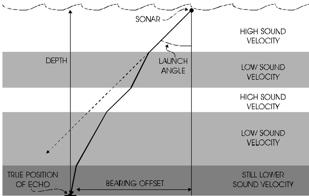
**Figure Chapter 4 - -32: Ray Tracing to Find the Bottom**
