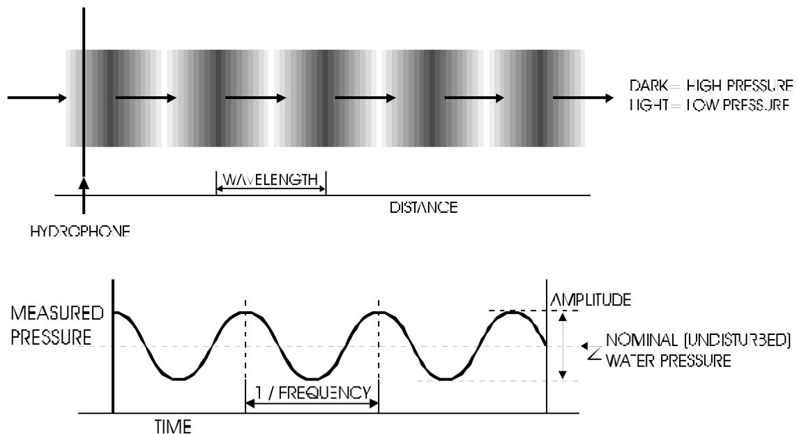
**Figure Chapter 2 - -1: Components of a Sound Wave**
