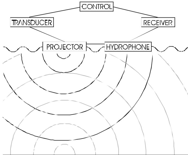
**Figure Chapter 5 - -2: Single-Beam Echo Sounding System**
