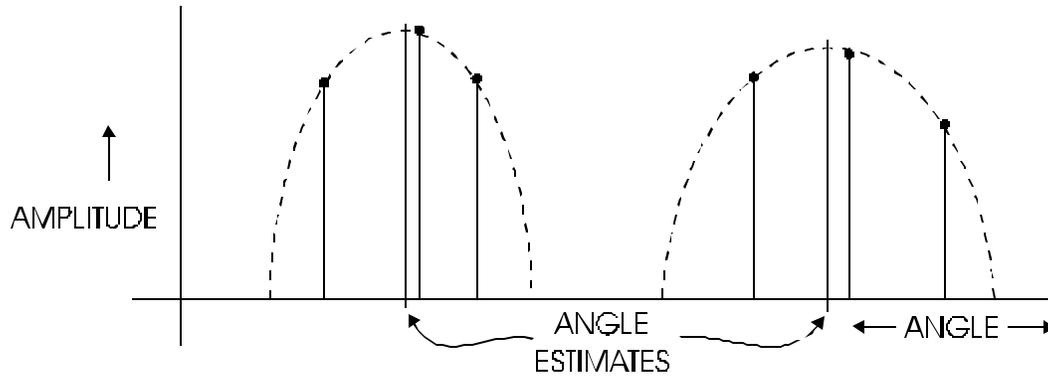
**Figure Chapter 4 - -11: Parabola Fitting for High-Resolution Angle Estimation**
