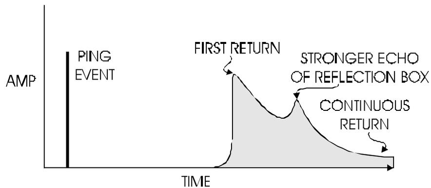
**Figure Chapter 5 - -7: Amplitude Versus Time Sequence**
