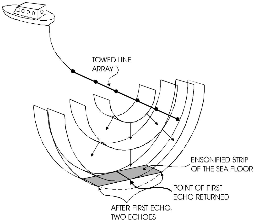
**Figure Chapter 5 - -9: Survey Vessel Towing a Line Array**
