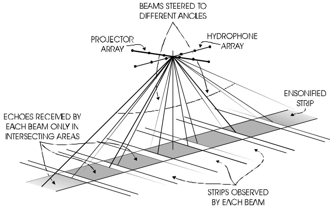
Figure Chapter 3 - -21: Mills Cross with Multiple Steered Beams
