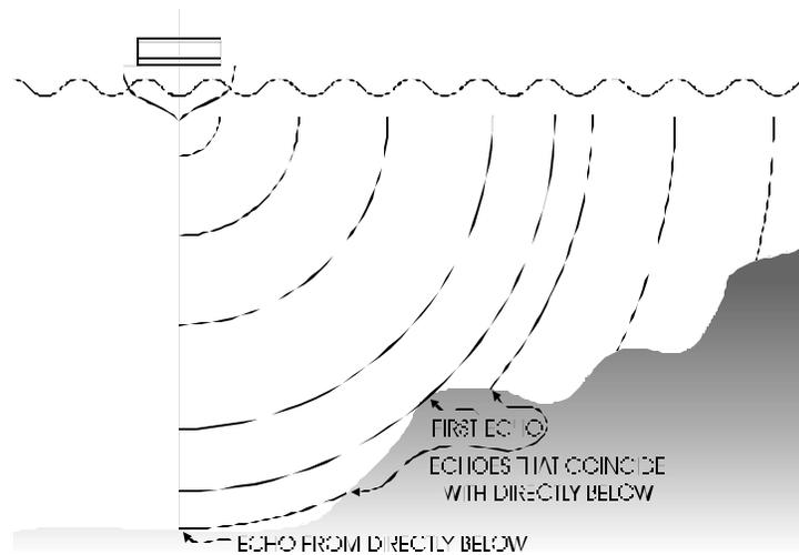
**Figure Chapter 5 - -14: Half of a Two-Hydrophone Sidescan Sonar**
