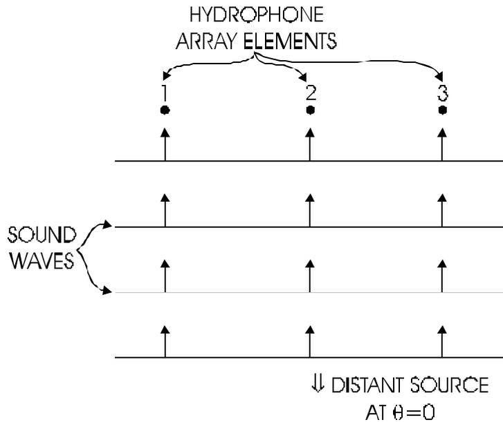
**Figure Chapter 3 - -9: Hydrophone Array with a Perpendicular Source**
