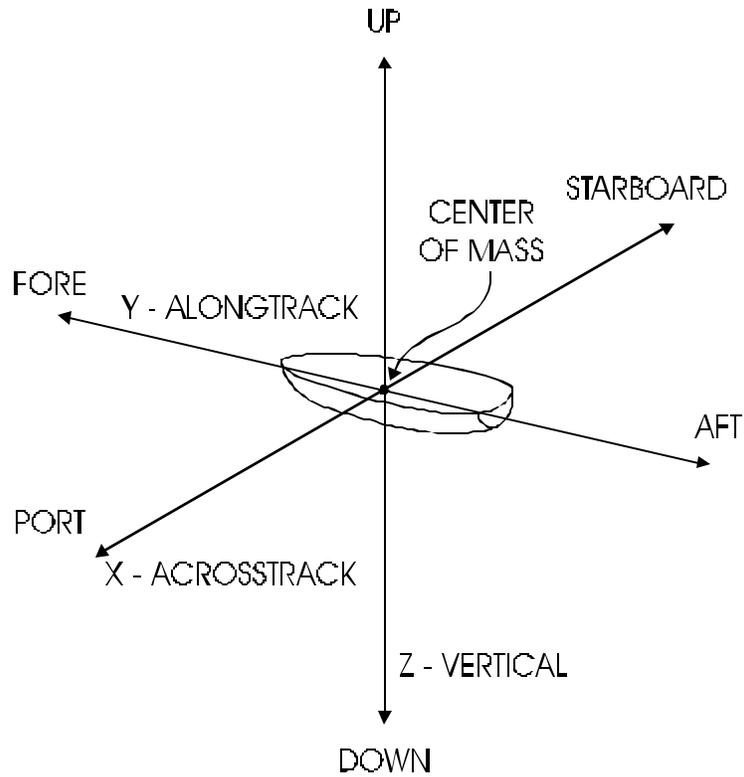
**Figure Chapter 4 - -12: Ship-Motion Coordinate System**
