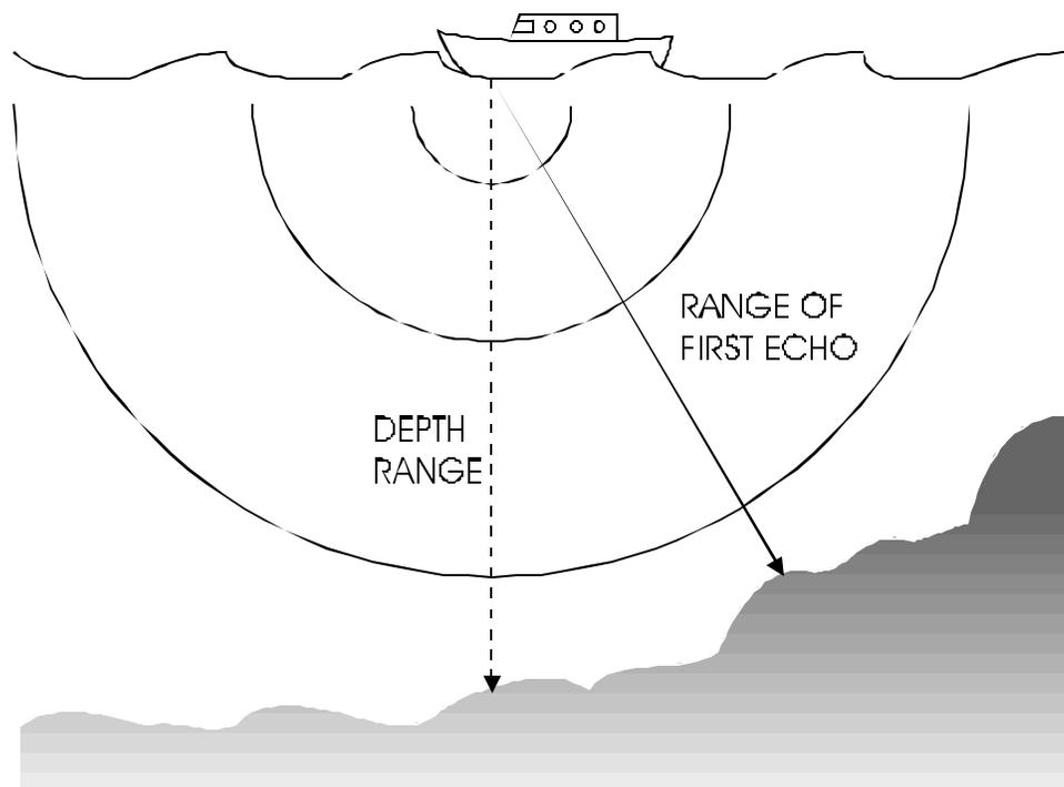
**Figure Chapter 2 - -5: Surveying an Irregular Sea Floor**
