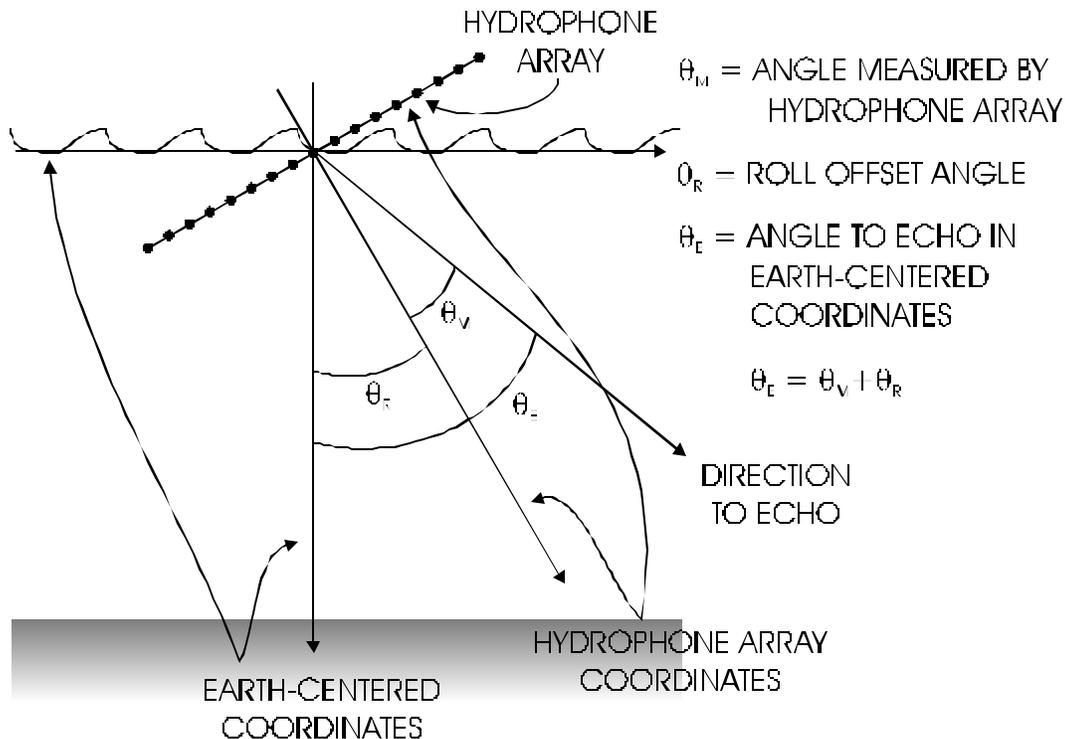
**Figure Chapter 4 - -15: Adjusting Measured Angles for Roll**
