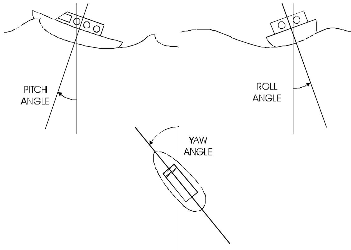
**Figure Chapter 4 - -14: Roll, Pitch, and Yaw Angles**
