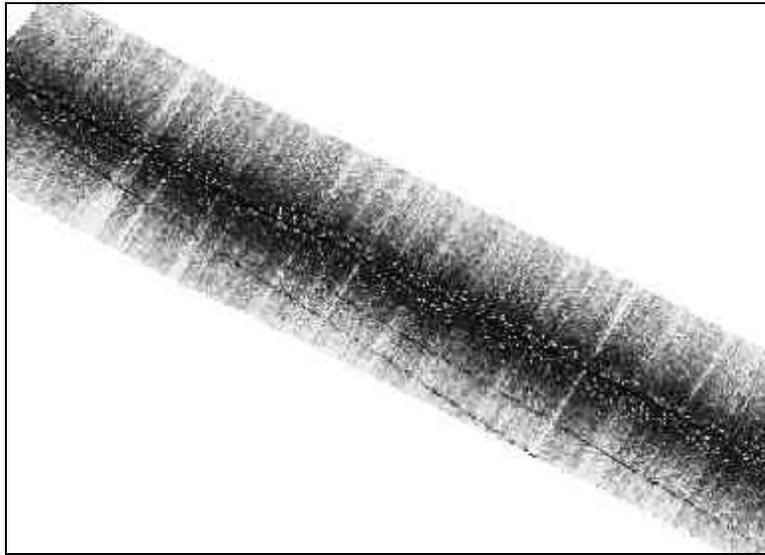
**Figure Chapter 5 - -13: Undersea Pipelines Detected Using Sidescan Sonar**
