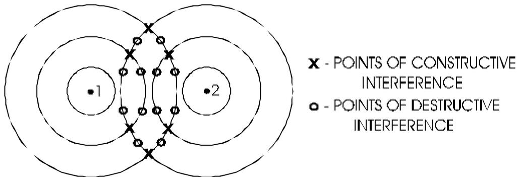
**Figure Chapter 3 - -2: Constructive and Destructive Interference**
