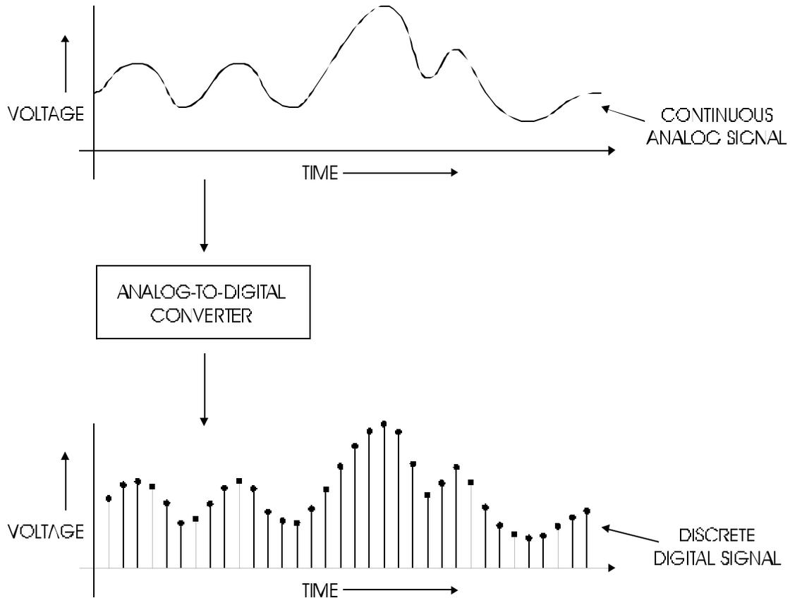
**Figure Chapter 4 - -1: Analog-to-Digital Conversion of Hydrophone Data**
